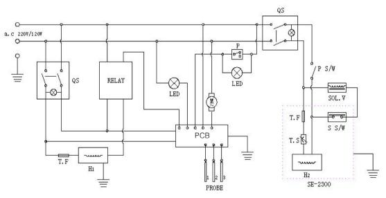
QS: power switch PCB: Pcb board
